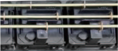
Integration welding of copper bar
