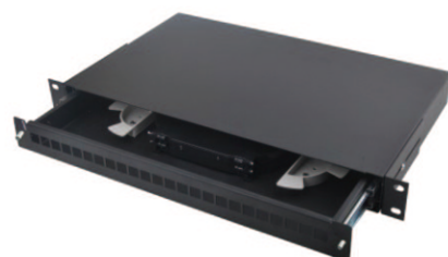
SWFO-0324 19-inch 24 ports drawer type,easy to operate available for simplex SC,FC,ST,LC adapter. Dimension(mm):482*260*1U
