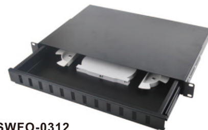
SWFO-0312 19-inch 12 ports drawer type,easy to operate available for duplex SC,FC,ST,LC adapter. Dimension(mm):482*295*1U
